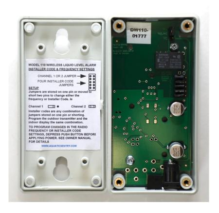
FIG 1 Indoor Alarm Display Interior
