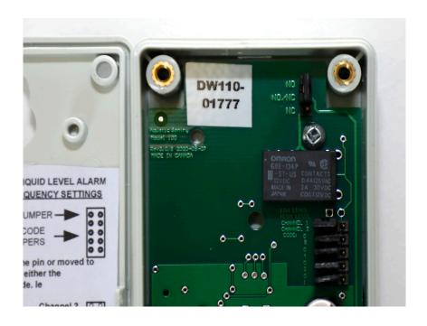
FIG 6 Indoor Alarm Display Setting relay to Normally Open or Normally Closed
